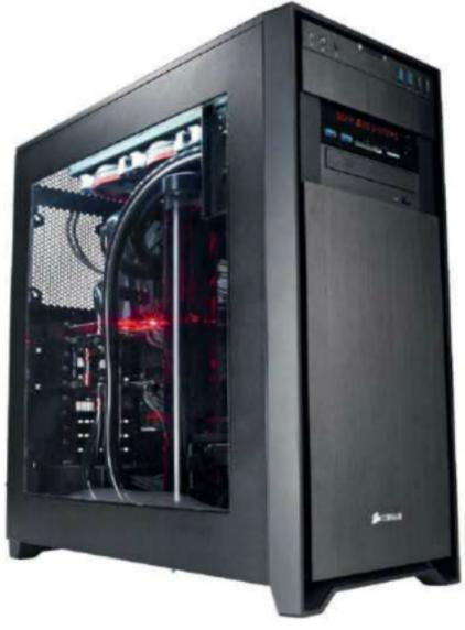
core speed boosted from 863MHz to 963MHz, and the memory from 6GHz to 6.2GHz (effective). To match the lighting and red Asus RoG logos on the motherboard, Scan has also picked red Monsoon compression fittings for the black tubing and EK blood red coolant. Finally, the pump of choice is a Laing DDC, which has a huge EK-RES X3 reservoir tube mounted directly on top, showing off the blood-red coolant.
