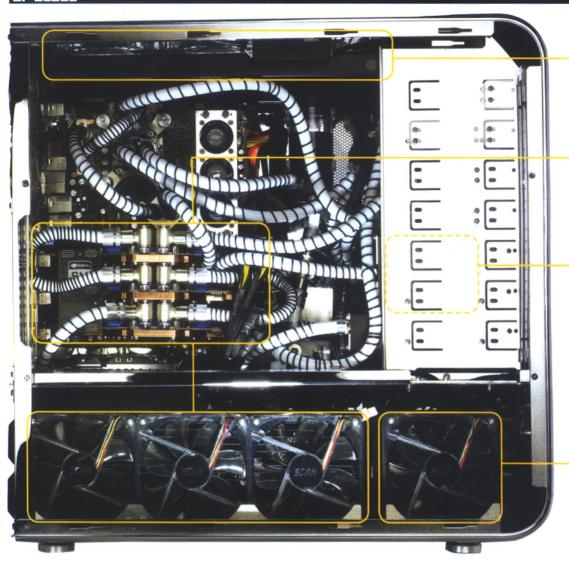
Scan modified the roof of the case, making space for a triple 120mm-fan radiator for the CPU.
