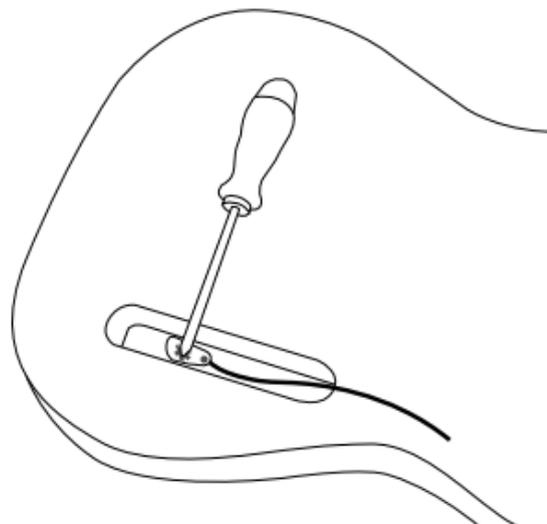
**NOTE:** Use a screwdriver to remove ground lug and screw from cavity. Remove lug and solder ground wire to Control Module as shown.
