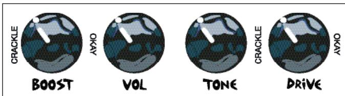
**BOOST:** Sets the boost level, which is engaged with the left stomp switch. [Start around 11:00 o'clock]. The Drive and Boost controls are based on my original Super Hard On™ gain control, so they may crackle when turned. This is perfectly normal.
