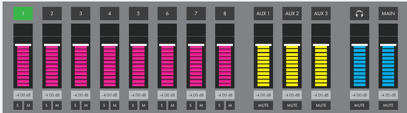
You can see the fader section is laid out like a traditional mixing environment. Each of the 8 input channels and each of the 5 output pairs (mains, aux 1-3, phones) have their own fader, channel select, and mute button. A solo button is also available on each of the input channels; soloing the outputs is not supported.
