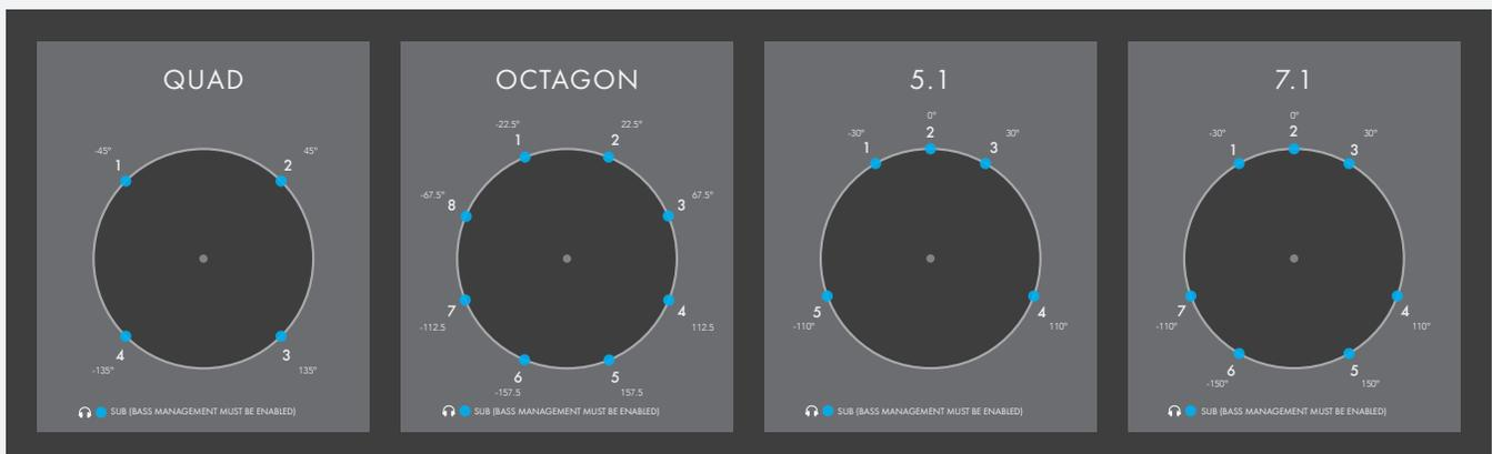
All surround formats begin with speaker 1 at the front-left position and increment clockwise. This may run contrary to established 5.1 and 7.1 film standards, but it makes plugging output channels into the appropriate speakers much easier.
