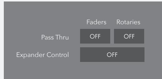
Pass Thru is meant to solve this. When both are enabled, faders and rotaries will not move until your finger “passes through” the current value. This will prevent any discontinuous jumps that may occur otherwise. You can enable pass thru for faders and rotaries separately if you prefer.
