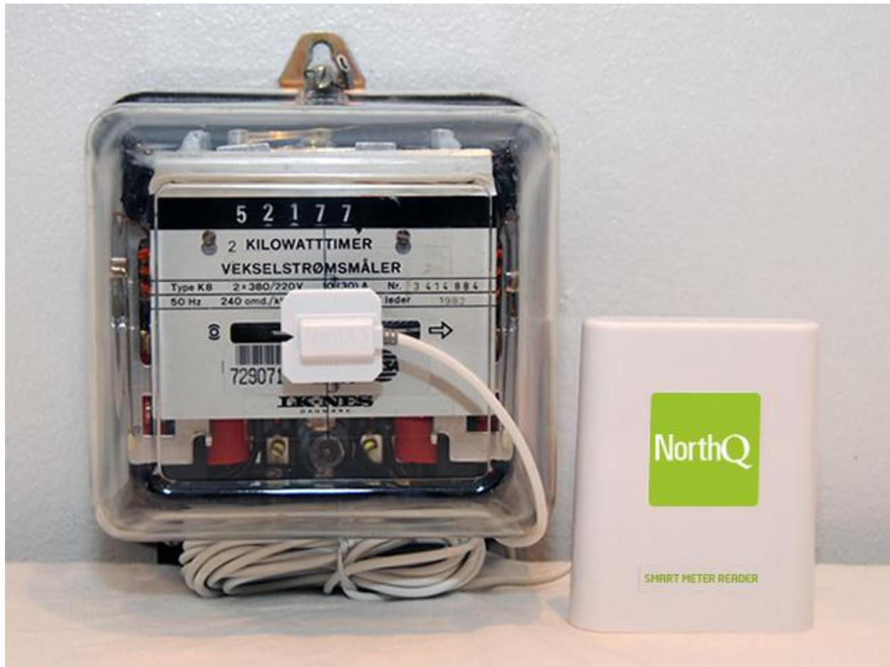
Figure 6 NorthQ PowerReader mounted on a mechanical meter
