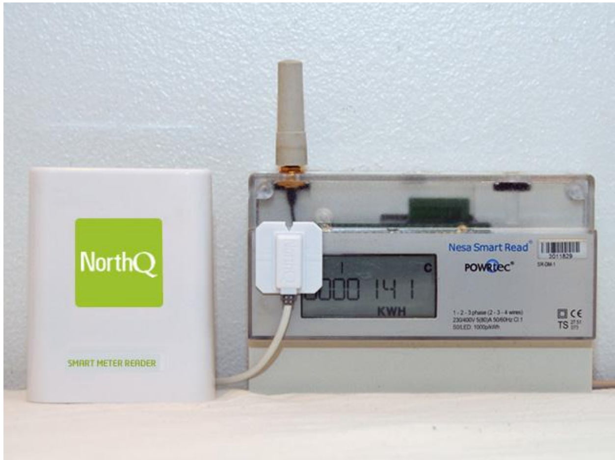
Figure 7 NorthQ PowerReader mounted on an electronic meter
