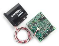
Enabling the onboard cache on a RAID controller card significantly enhances performance — especially in RAID 5 and RAID 6 scenarios — by accommodating both read caching and write caching of data. But data stored in the cache for write caching can be lost if the cache is not protected against a power or system failure.
